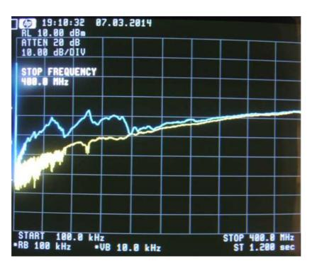
A small attenuation of 10 to 15dB is measured in low frequencies, up to 180MHz. Attenuation is close to 0dB for upper frequencies up to 2GHz at least.
