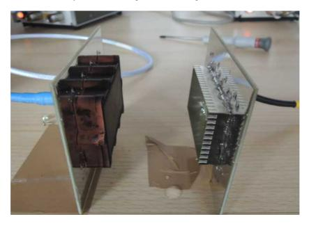
Once again, no significant shield efficiency was measured for frequencies above 200MHz. However for lower frequencies a reasonnable shield efficiency was measured, ranging from 5-8dB (<80Mhz) to 10-15dB (80Mhz to 200MHz) :
