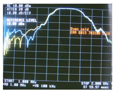
No significant shield efficiency was measured for frequencies above 200MHz. Even a negative efficiency was observed from 200 to 300MHz, probably due to multipath effect on the test setup. A 10dB attenuation is measured for lower frequencies
