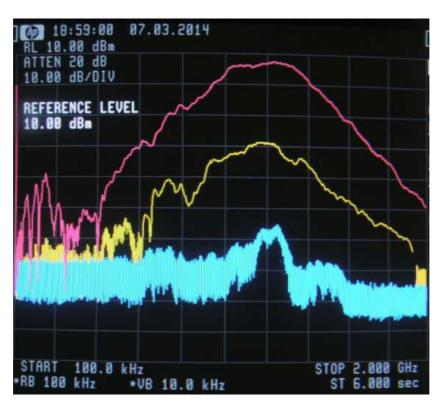
An overall 5dB degradation in the shield efficiency is measured from 200MHz upward.
