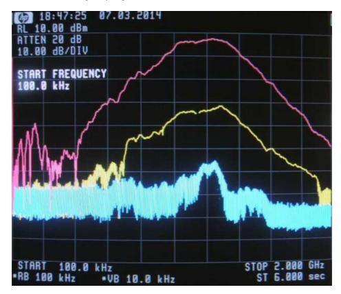
The measured attenuation in this optimal configuration is then around 25 to 30dB from 400MHz to 1,5GHz, down to 20dB up to 2GHz and at low frequencies.
