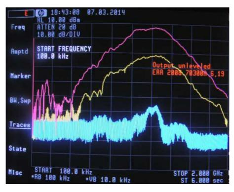
(pink : reference without any shield, yellow : with shield in place, blue : sensitivity baseline measured with a 50-ohm load in place of the transmitting antenna).
